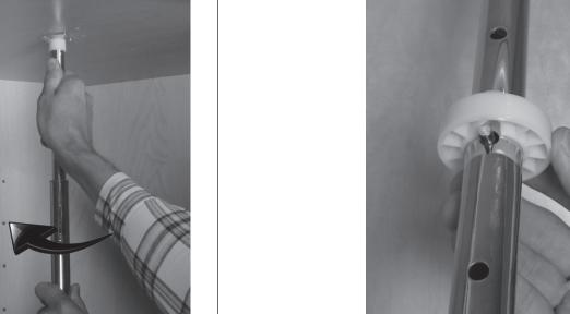
Holding onto the lower pole, twist the upper pole counter-clockwise to release. Extend pole upwards until it rests firmly against the Top Mounting Bracket and tighten by turning the upper pole clockwise.
