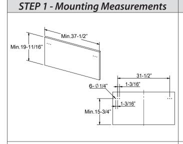
Determine the mounting location for the Smart Rail Storage Solution and layout mounting location on the wall as shown above.
