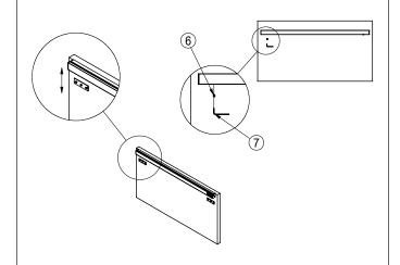
Place the notch in the rear of the hang rail over the cleats and install the Allen set screws. Tighten with the provided Allen wrench.
